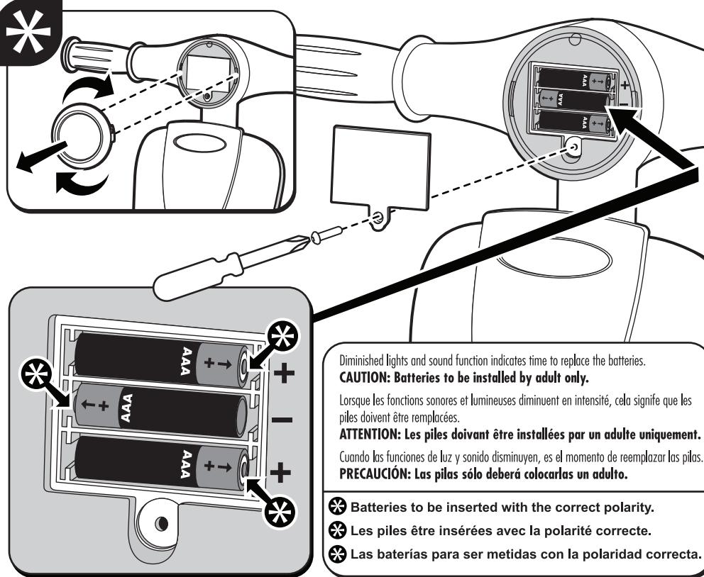
Requires 3 "AAA" (called LR3 in some countries) batteries. Install new batteries as shown in the polarity diagram (+/-) inside battery compartment.
